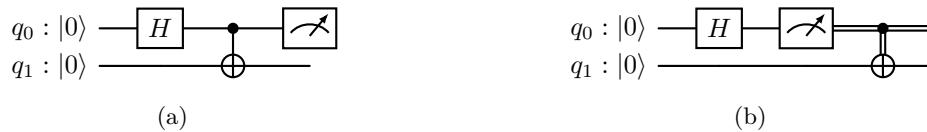
Figure 2.4: Two equivalent circuits showing the deferred measurement principle: a measurement on q_0 can be postponed and replaced with a classically controlled operation on q_1 .
