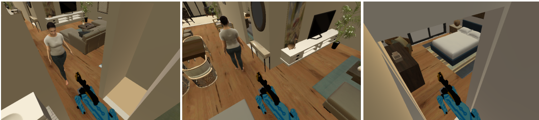
Fig. 3.7: Three unsafe scenarios from the Habitat Lab experiments: On the left, the humanoid approaches the robot, which should move backward to avoid collision. In the center, the humanoid moves away, and the robot should follow while avoiding obstacles. On the right, the humanoid approaches from behind, and the robot should turn to avoid an unexpected collision while searching for the humanoid.
