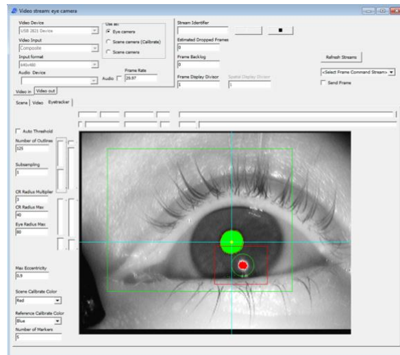
Figure 12. Example of the user-view from the MoBIGaze eye-tracking system. The pupil is highlighted in green. The little red dot underneath is the corneal reflection, projected from the eye-tracker into the participant's eye (from https://sccn.ucsd.edu/ ).
