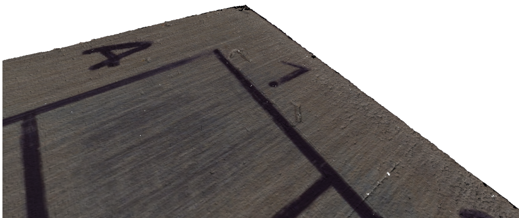
Figure 6.11: Part of the silver sample reconstructed using the data from the conoscopic holography scan and a texture obtained fusing multiple photos taken with a Nikon D810.
