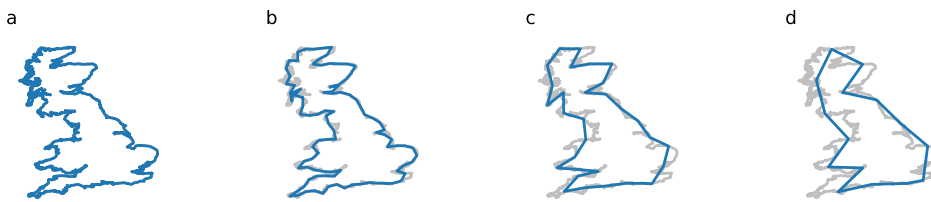
Figure 5.17: Application of the algorithm proposed by Richardson using a radius (divider spacing) of: a) 80 m, b) 40 km, c) 100 km, d) 160 km. Superimposed to the coastline of Britain.
