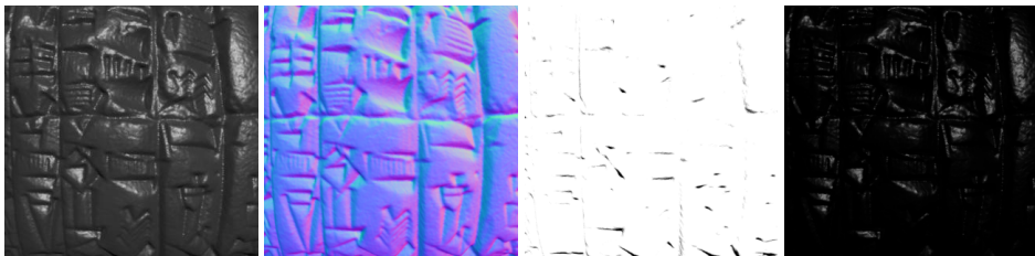
Figure 3.5: Rendered multi-light image collections (a) come with associated normal maps (b) that can be used for Photometric Stereo algorithms evaluation, shadow maps (c), that can be used for shadow detection testing and specularity maps (d)
