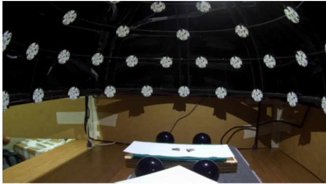
Figure 1.3: A multispectral light-dome based acquisition setup by Ciortan et al. [24]
