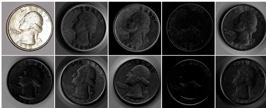
Figure A.18: Image sample (top left) and the nine NeuralRTI encoded byte planes represented as greyscale images for a coin RTI encoding
