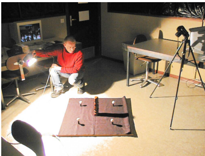
Figure 1.1: An hand-held light acquisition setup by Masselus, et al. [83]
