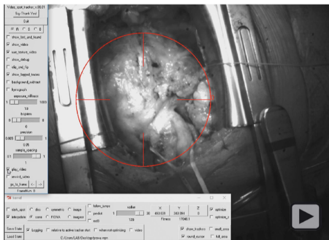
Video 1: Intraoperative video recording of cardiac kinematics of the right ventricular outflow tract. A virtual target (red) allows to focus the virtual marker. The virtual marker (yellow) on the first frame of the video follows the light spots on the epicardial surface, tracking the spatial-temporal coordinates x , y and t of that marker in each frame.
