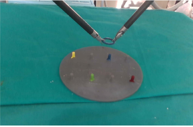
Fig. 6. Dual arm manipulation experiment. The two arms carries a ring while performing circular trajectories through the workspace.
