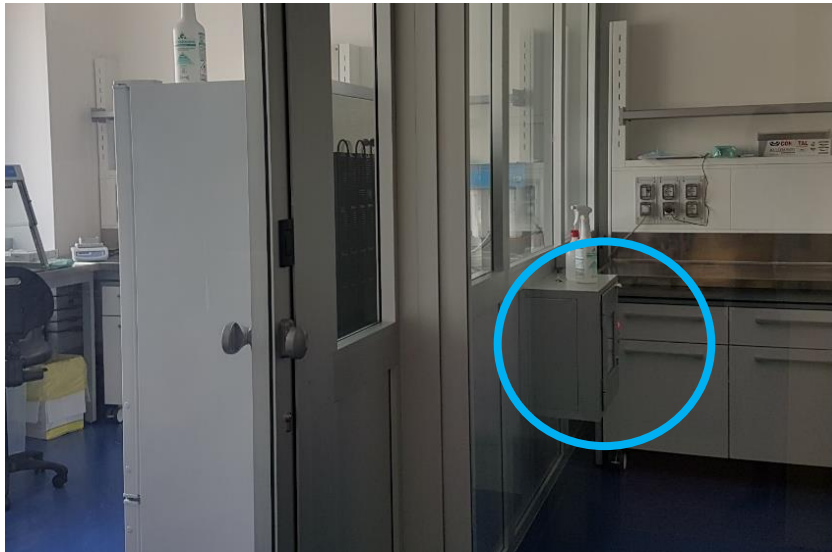
Figure 10. Picture of the “pass-through cabinet” to preserve the sterility of the specimen during manipulation steps
