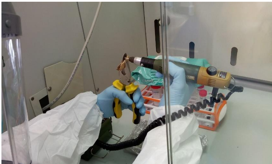
Figure 8. Drilling and pulverization of a rib specimen
