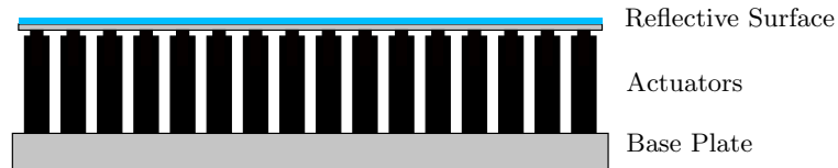
Fig. 2.8: Stacked array DM. The actuators, attached to the base plate, move longitudinally and shape the reflective surface.
