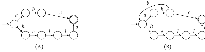
FIGURE 6.2: (a) A_1 , \mathcal{L}(A_1) = \{abc, hello\} . (b) A_2 , \mathcal{L}(A_2) = \{abc, hello\} \cup \{(abb)^n \mid n > 0\} .
