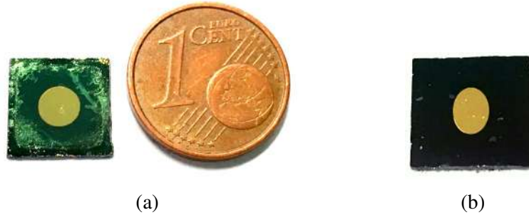
Figure 5-15: Fabricated membrane mirrors with circular (a) and elliptical (b) boundary (1 euro cent coin as size reference). OBS: The picture of the circular mirror has been taken after experimental characterization with this sample, which is why the edges of the nitride layer are scratched.
