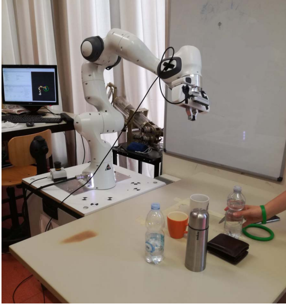
Fig. 1. The operative scenario. A robot is asked to actively recognize and localize all the objects on a table top.
