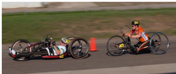
Figure 1.8. Recumbent handbike (on the left) and knee-seat handbike (on the right) ( http://www.sports.org.au/cycling/ ).
