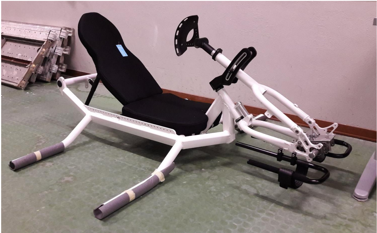
Figure 3.8. The physical prototype of the frame for the HWB v. 2.
