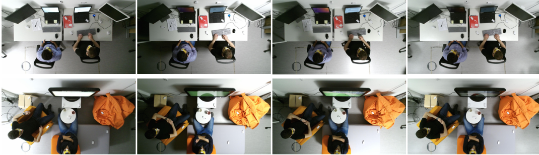
FIGURE 7.5: Illustration of 4 illumination variants within the two rooms. From left to right, the images illustrate the illumination provided by 1, 4, 7 and all 8 luminaires switched on in the two scenes.
