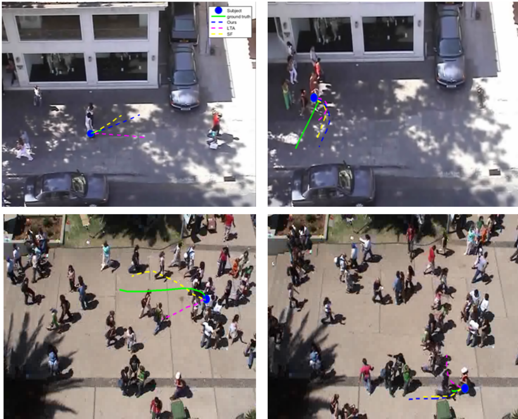
FIGURE 6.4: Illustration of common failure cases of trajectory forecasting. Acceleration, deceleration and static groups are common failure cases across all approaches.
