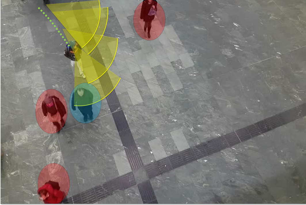
FIGURE 6.7: VFOA pooling: For a given subject, he will try to avoid collision with the people who are inside his view frustum (blue circle). Others (red circle), will not influence his trajectory as they are no in his view frustum.
