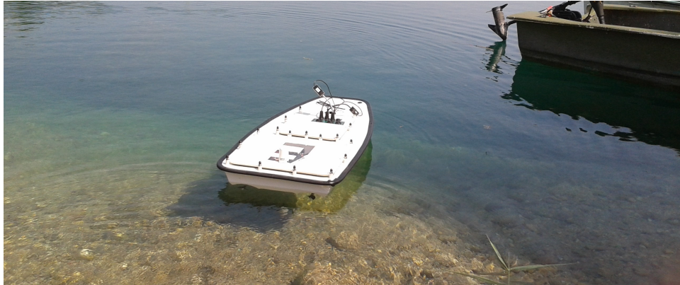
Figure 1.1: Mobile platform that we used: Platypus Lutra equipped with pH, dissolved oxygen, temperature and electrical conductivity sensors. The computation is on board and performed by an Arduino Due and a smart-phone.
