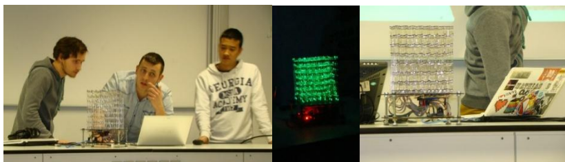
Figure 10. Luminous cube realized with micro controller.
