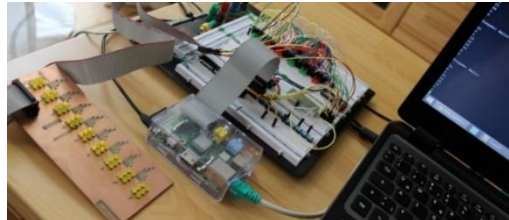
Figure 8. E-book-reader with Braille lettering output.
