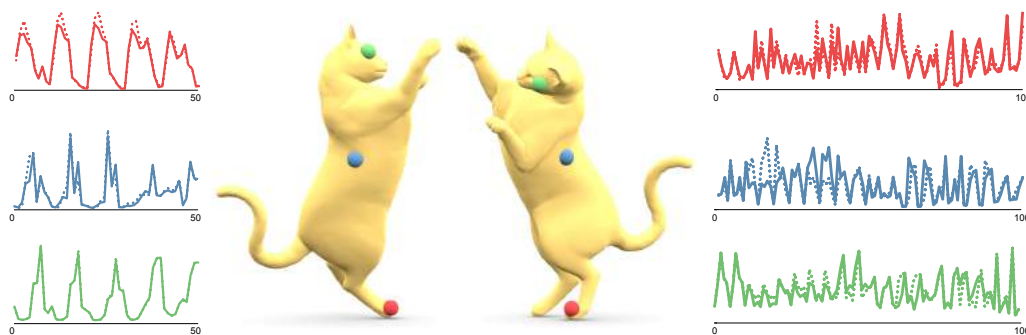
Fig. 5.15: Comparison between WFT (left) and AWFT (right) descriptor computed at three symmetric points of the cat shape (points and corresponding curves are color-coded). Solid and dotted curves represent descriptors of points from the left and right side of the cat, respectively.
