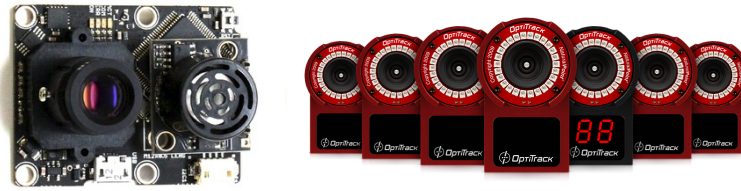
Figure 6-6: The Px4Flow visual odometry device and the OptiTrack system. Credits: www.optitrack.com
