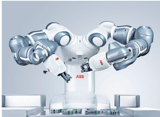
Figure 1-1: Robot Yumi ABB: a popular robot used in industry mainly to assemble light products. Credits: www.abb.com
