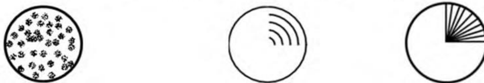
Figure. 1.21 Sketch indicating radial, concentric and random carbon layer orientations in CSs.
