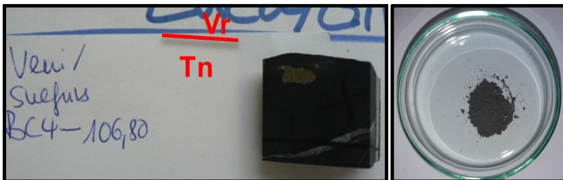
Figure 6.2 Optical images of sonic drilled black shale core (left) and of the powdered sample (< 80 \mu\text{m} ) of the carbonate shale (right).
