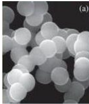
Figure 1.16: HRSEM image of carbon nanopearls via CVD process [7].
