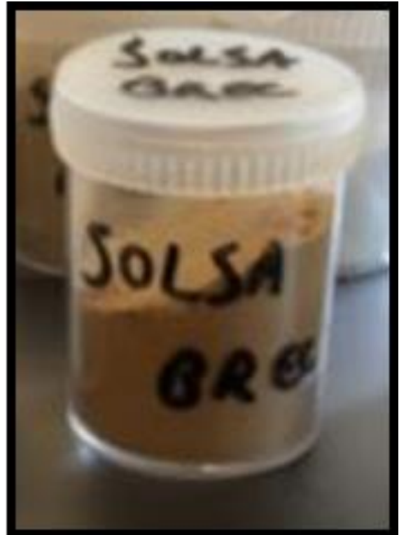
Figure 5.2 Optical images Sonic drilled cores breccia (left) and the powdered sample ( < 80\mu\text{m} ) of the breccia (right).
