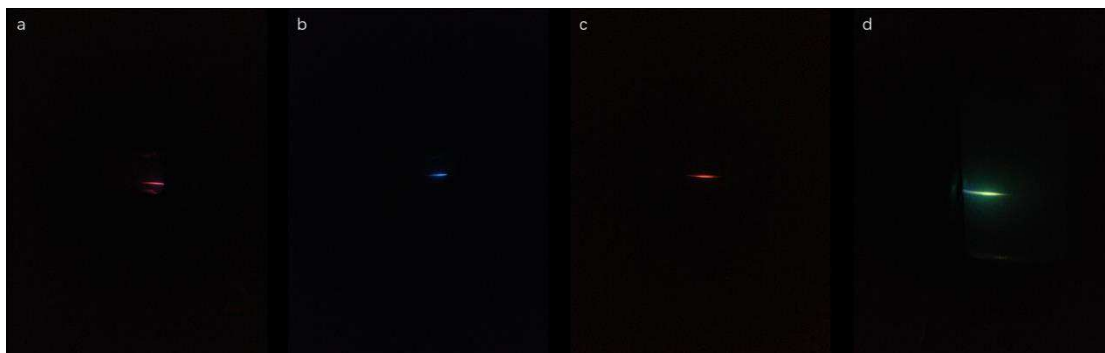
Figure 8.13 UC emission image for NaGdF 4 :Yb,Tm@NaGdF 4 :Eu/Tb NPs (a, b) and KGdF 4 :Yb,Tm@KGdF 4 :Eu/Tb NPs ( \lambda_{ex} = 980 \text{ nm} ).
