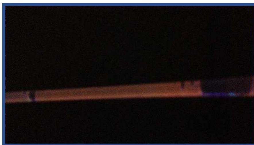
Figure 7.8 Red emissions of transparent CuSRs solution at higher temperature (>150°C). This emission disappears and transparent solution becomes milky when it cools down.
