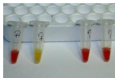
Fig. 36 Rapid Carba NP test home-made. On the left positive result, on the right negative result.
