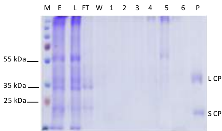
Figure 4 SDS-PAGE and Coomassie staining on 12% polyacrylamide gel of 14 \mu l of the following samples: total protein extract (E), sample loaded on anion-exchange chromatography (clarified sample) (L), Flow through (FT), wash (W), elution steps (1-6) done with NaCl gradients from 50 mM to 1 M, 4 \mu g of purified unmodified CPMV eVLPs as positive control (P). The Rubisco's subunit molecular weight (55 kDa), the CPMV large and small coat proteins molecular weight (respectively 35 and 25 kDa) are indicated. M: molecular marker (PageRuler™ Plus Prestained Protein Ladder, Thermo Scientific).
