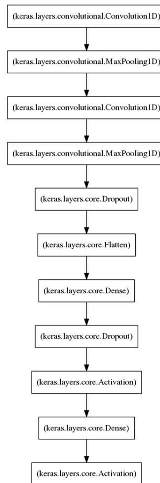
Figure 5: CNN architecture.
