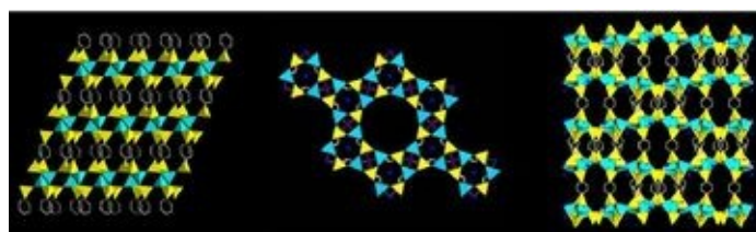
Figure 1. Structure of ECS-17 (left), ECS-14 (middle) and ECS-3 (right). [SiO 3 C] tetrahedra in yellow, [AlO 4 ] tetrahedra in cyano, Na ions in blue, phenylene ring in grey.
