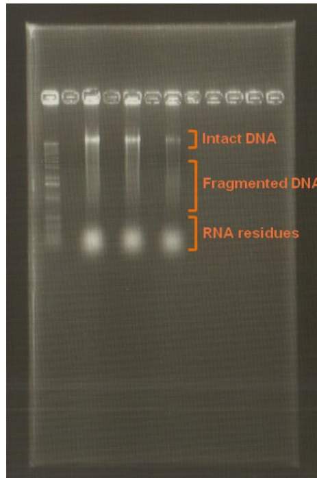
Figure 6: 1% agarose gel of DNA extracted by phenol-chloroform classical method.
