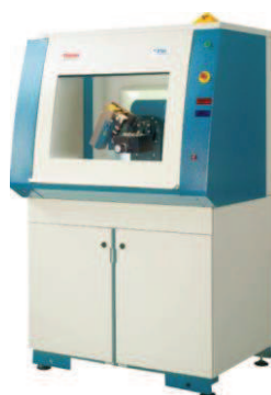
Fig. 3.4 X-ray powders diffractometer used for the characterization of the compounds of this thesis.
