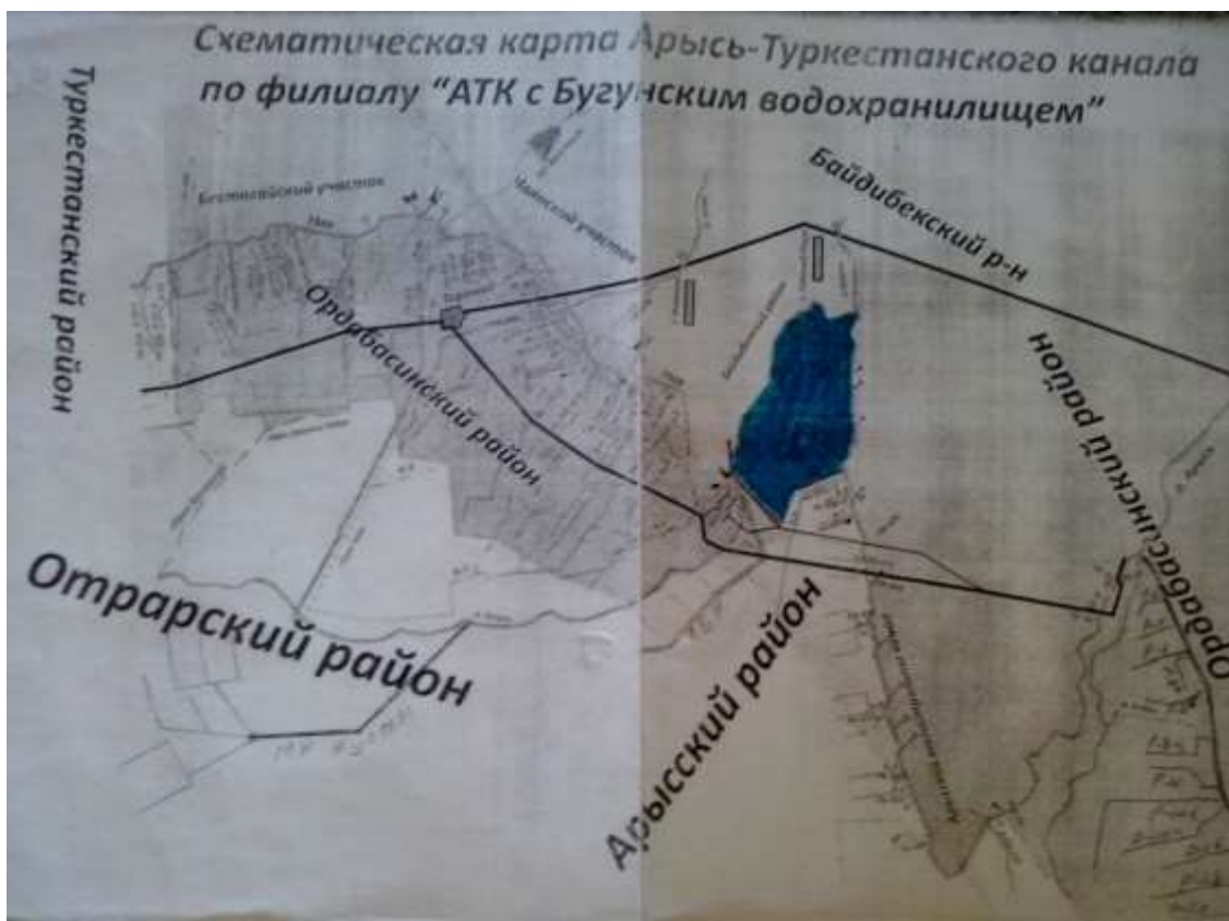
FIG. 47: Scheme map of the Arys-Turkestan irrigation system: on the right the Arys canal and the secondary level canals' system, in the centre the Bogun reservoir and in the right the Arys-Turkestan canal and the related irrigated area (source: South-Kazakhstan RGP).
