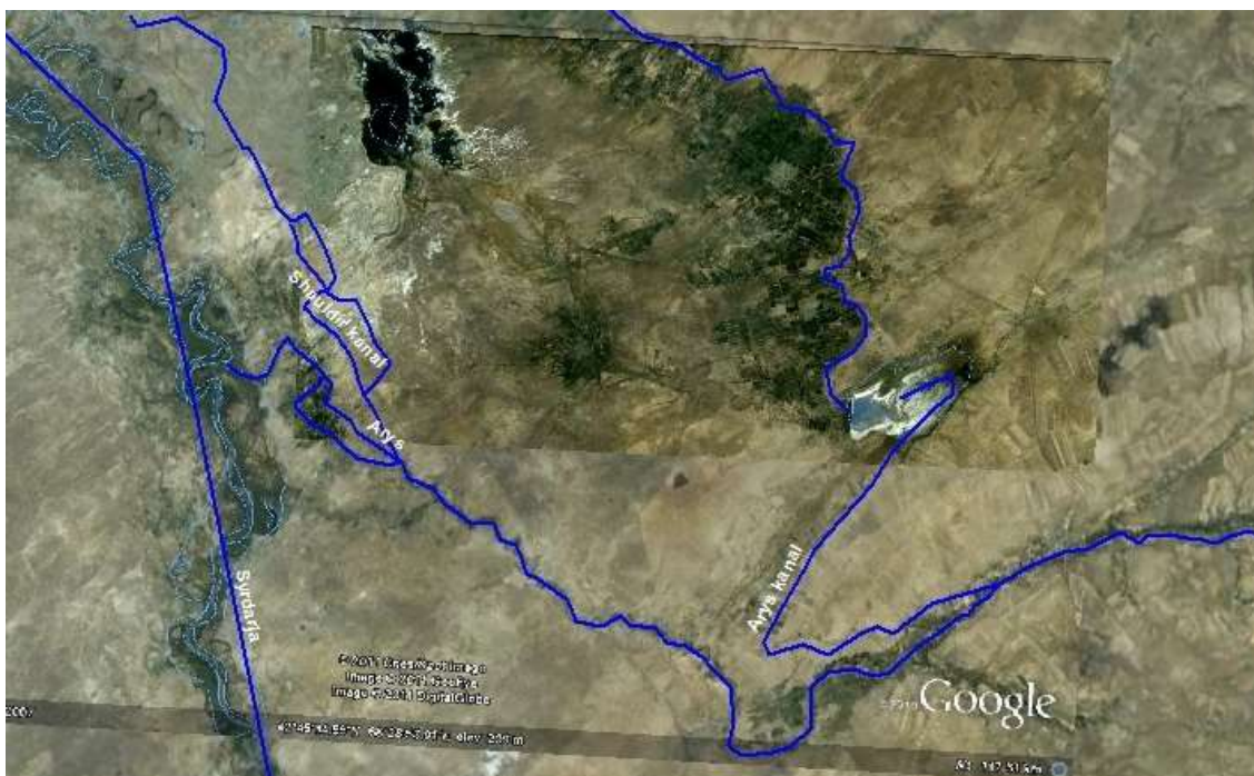
FIG. 44: GIS elaboration of an overlay of satellite images (source: Google Earth) representing the canals' system and the irrigated areas of the central-downstream side of Arys valley.
