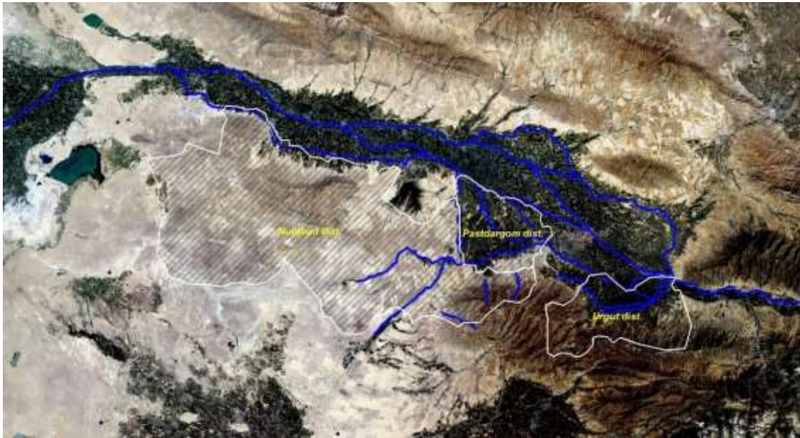
FIG. 6: GIS elaboration of a satellite image representing the Middle Zeravshan Valley' irrigation scheme (flowing from the E to the W) and the three districts selected for the field research. three districts selected for the field research.
