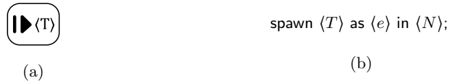
Fig. 5.25. (a) The spawn command creates a new process instance of type T returning a new identifier that can be stored into a variable. (b) The encoding of a spawn command.
