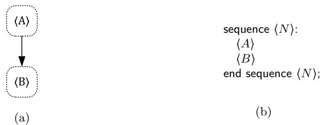
Fig. 5.15. (a) A sequence is represented by solid line between two blocks ending with an arrow. (b) The encoding of a sequence block.
