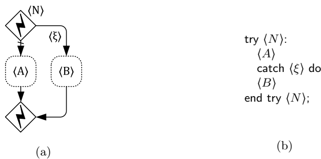
Fig. 5.19. (a) A try block with two branches: the first one is marked with an oblique segment and represents the default execution, while the second one is annotated with an exception identifier \langle \xi \rangle . (b) The encoding of a try block.
