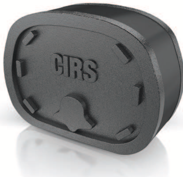
Figure 2.2: CIRS 057 interventional 3D abdominal phantom.
