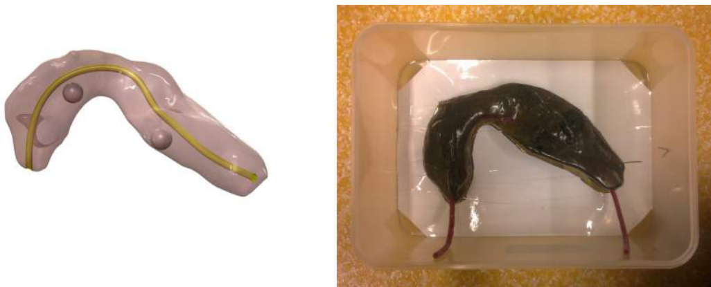
Figure 3.2: The CAD model for the realization of the phantom (left) and the pancreas phantom (right) with the internal duct.
