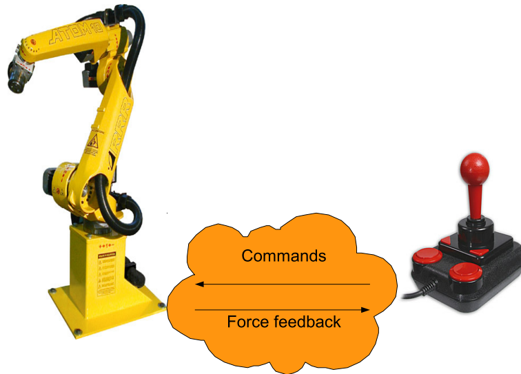
Fig. 7.6. Architecture of a networked control system.
