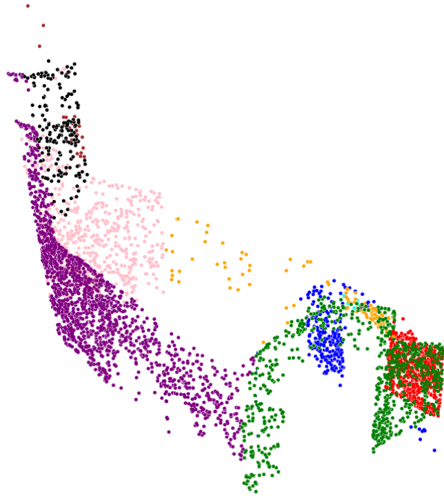
Fig. 5.2. Planes recovered by model fitting. The colour of the point encodes the plane it belongs to.
