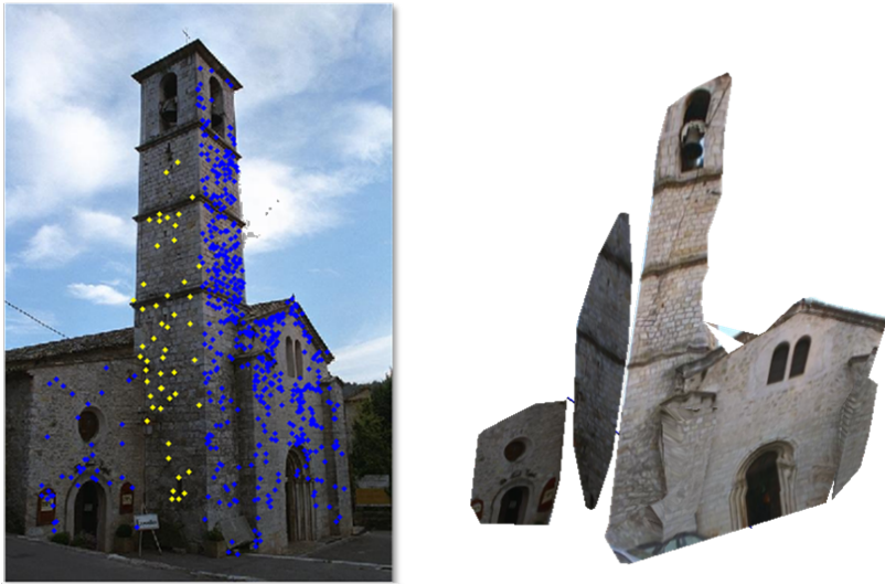
Fig. 4.7. The clustered point cloud and the corresponding triangulated model.
