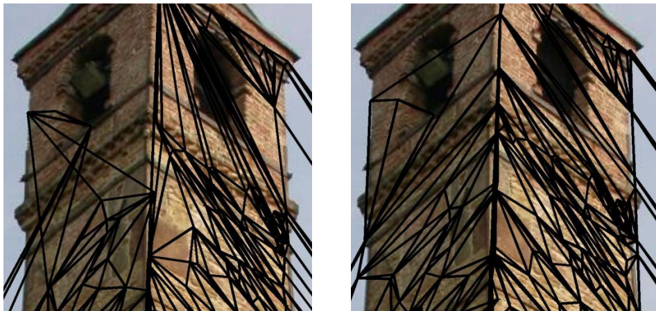
Fig. 5.3. Detail of the triangulation before (left) and after (right) augmentation with boundary points.
