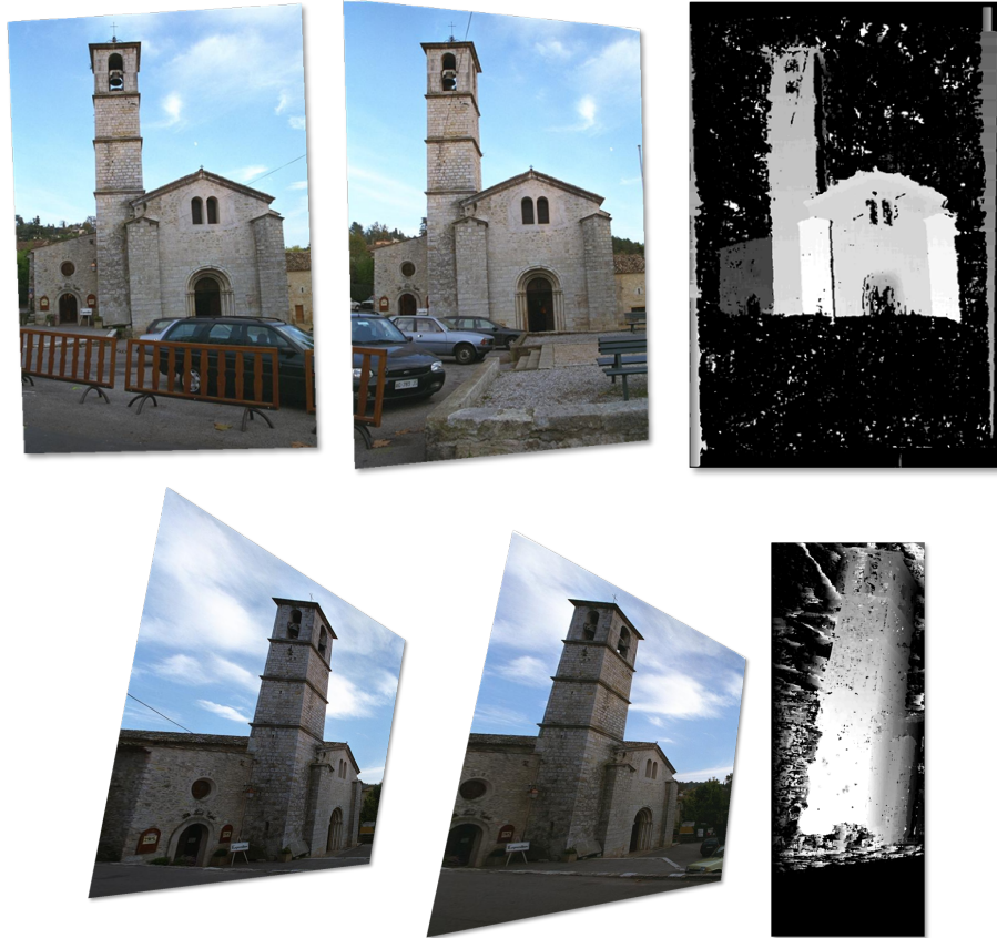
Fig. 4.6. The first two couples automatically recovered by the proposed view selection heuristic and the corresponding (left) disparity map.
