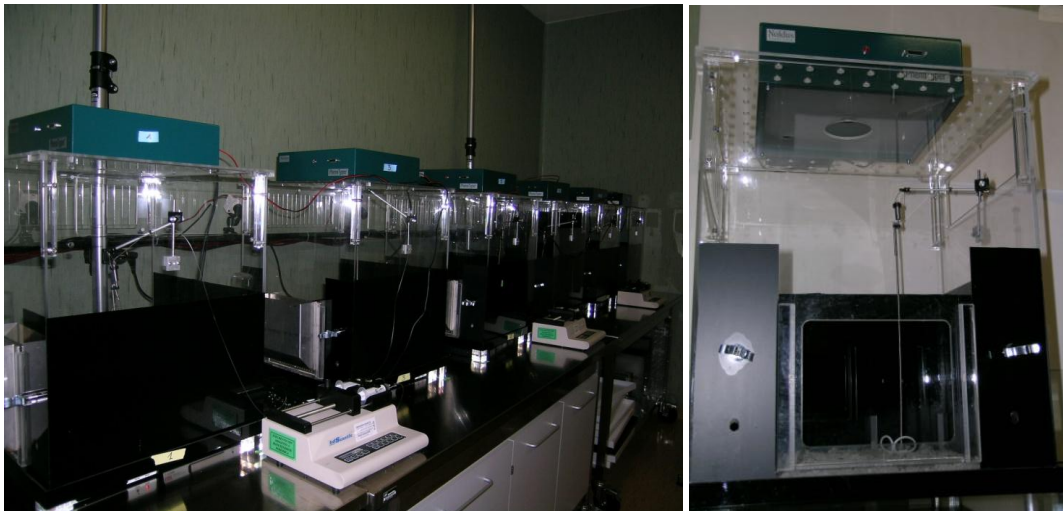
Figure 51: The PhenoTyper Cages with infusion pump and blood bleeding equipment.
