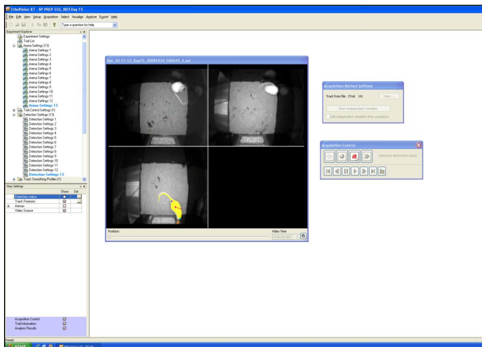
Figure 20: The automatic video tracking performed using EthoVision XT software on the multiplexed video signal which come from 3 Phenolab cameras top units.
