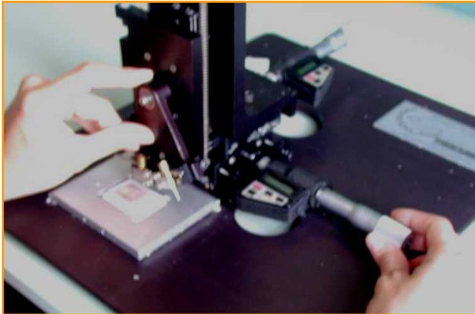
Figure 14. TMA building with tissue microarrayer, which allows to take a core of 1 mm diameter from donor blocks and put it in a host block
