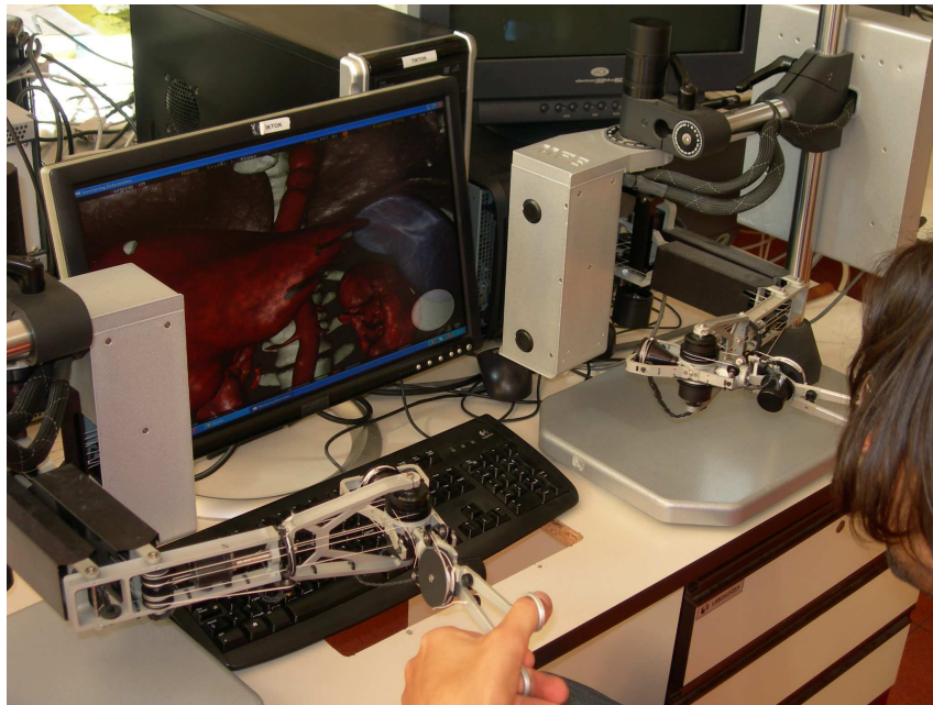
Fig. 8.1. The complete simulation setup: two haptic devices allow the user to interact with the virtual environment that is perceived through haptic feedback and with graphical rendering.
