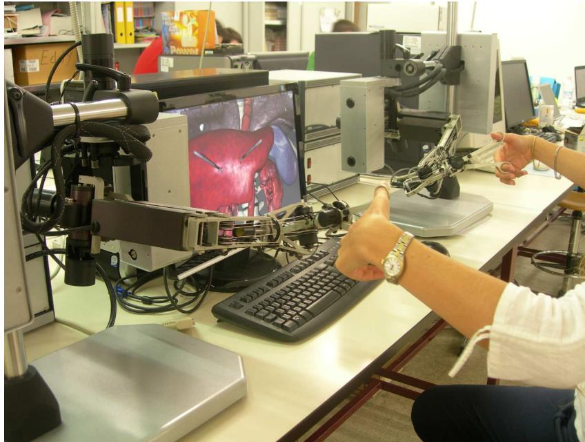
Fig. 7.17. The simulator experimental setup: haptic feedback is provided through two MPB Freedom 7s connected to the simulator, graphic rendering is obtained with the described method
