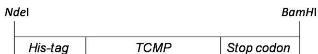
Figure 8. Schematic drawing of the construct for the expression of recombinant TCMPs. Restriction endonuclease sites used for the recombinant expression constructs are reported.
