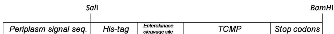
Figure 12. Schematic drawing of the construct for the expression of recombinant TCMP-2 in the periplasmic space. Restriction endonuclease sites used for the recombinant expression construct are reported.
