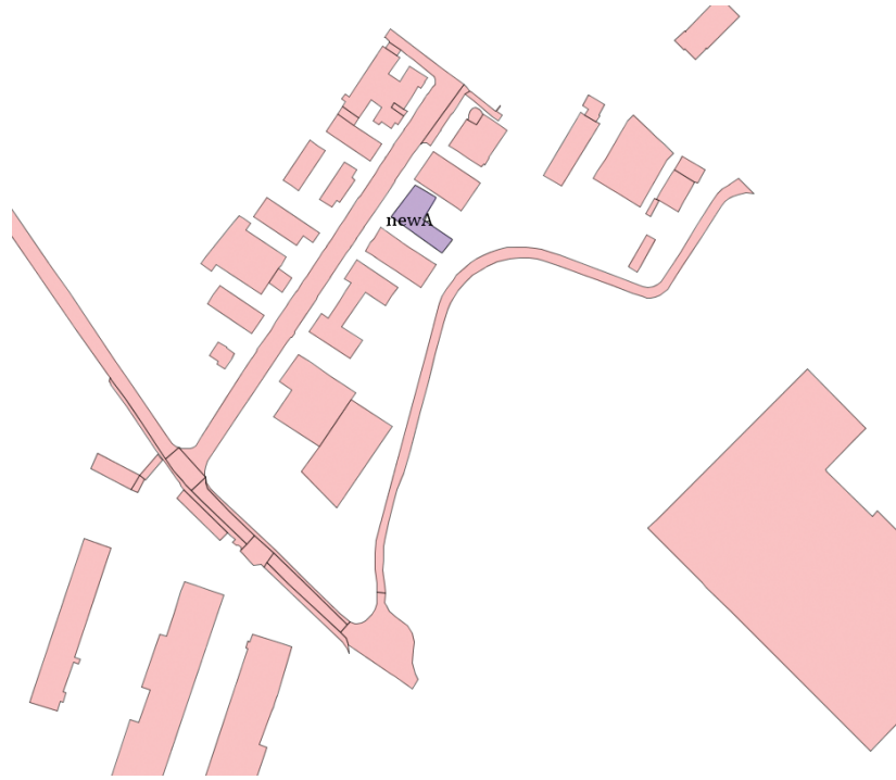
Fig. 4.18. The result of the integration performed with the proposed technique: the new building labeled with new_A is now perfectly inserted between the two surrounding buildings: thanks to the role covered by the accuracy of relative distances, the disjoint relation has been preserved.
