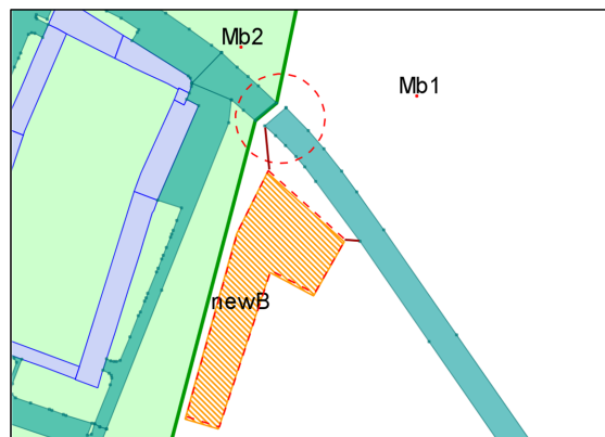
Fig. 1.8. Example of problem that may arise when an integration is performed locally without propagating its effects to the adjacent datasets. In particular, the road crossing the two dataset becomes disconnected, since only the portion laying in Mb_1 is modified.
