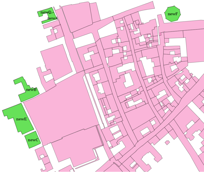
Fig. 4.20. The result of the integration performed with the proposed technique: the new buildings labeled with new_A - new_F are now perfectly integrated with the surrounding street areas: thanks to the role covered by the accuracy of relative distances, the disjoint relations have been preserved.
