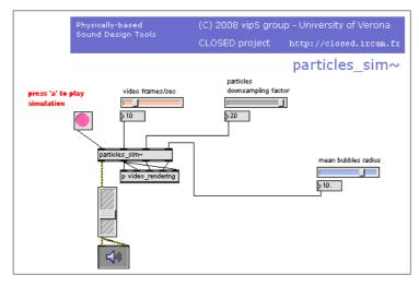
Fig. 2.15. The Max/MSP patch implementing the particle model for fluid simulation.
