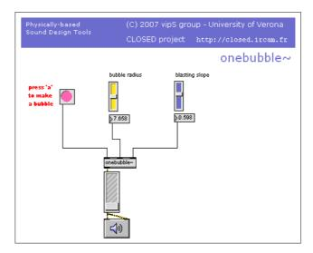
Fig. 2.5. A Max/MSP patch making use of the single bubble model, implemented as the *external* named onebubble $\sim$ .
