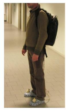
Fig. 3.9. The complete interface, with the early version shoes prototype. The backpack hosts a laptop and an acquisition board which senses data from the shoes. These data drive a set of real-time physically-based models running on the laptop and providing low-latency audio feedback through the shoe-mounted speakers.
