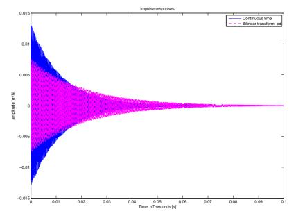
Fig. A.2. Impulse responses of a continuous-time and the bilinear transform-ed harmonic oscillator having natural frequency  $\omega = 12000$  Hz, damping coefficient g = 166.6667 Hz and modal mass m = 0.001 Kg. The sampling frequency is  $F_s = 44.1$  kHz. It is clear that the damping  $g_{BT}$  and the modal mass  $m_{BT}$  of the discretized oscillator are respectively lower and greater than the original continuous time versions g and  $m_{BT}$ .
