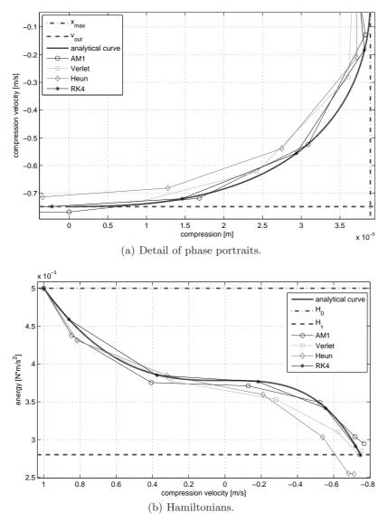
Fig. 1.8. Comparison of phase portraits and Hamiltonians for different implementations of a simulation example following *case 2*. The values of parameters are the same as in Fig. 1.1 with  $v_{\rm in} = 1$  m/s. The contact time equals 6 samples.
