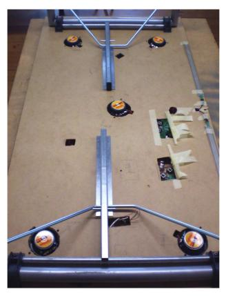
Fig. 3.4. The underside of the Gamelunch, showing the holes hosting the five loudspeakers and the two game-pad's circuit boards.
