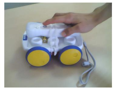
Fig. 3.5. The toy trolley mounting a Wii Remote controller, which is used as input interface for the game.
