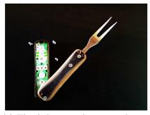
(a) The fork, opened up in order to show the embedded board which is taken from a Wii Remote controller.
