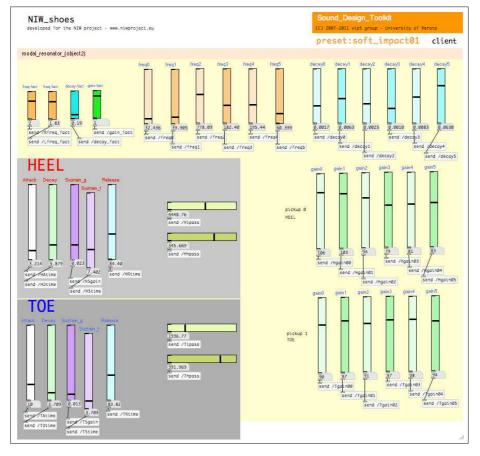
Fig. 2.7. Pd example patch implementing the soft impact model. On gray background are the controls for the envelopes and filters processing the noise burst, while on light orange background are the controls for the modal resonator.
