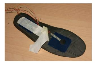
Fig. 3.8. The insoles with two sensors applied, respectively in correspondence to the tip and the heel. Each sensor is covered with a thin rigid plastic layer which allows to decouple the sensor's area from its exact location on the insole.
