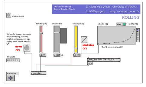
Fig. 2.10. The main Max/MSP example patch for the rolling model. The velocity map represents the acceleration/deceleration curve, which can be drawn by the user. A number of preset curves are provided, and new ones can be saved and recalled.
