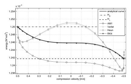
Fig. 1.7. Comparison of Hamiltonians for different implementations of a simulation example following *case 1*. The values of parameters are  $k = 10^7 \text{ N/m}^{\alpha}$ ,  $\mu = 0.01 \text{ s/m}$ ,  $\alpha = 1.3$ ,  $v_{\text{in}} = 0.5 \text{ m/s}$ . The contact time equals 19 samples.
