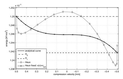
Fig. 1.10. Comparison of the Hamiltonians of a Heun-based simulation example following *case 1*, with and without corrections.
