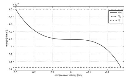
Fig. 1.4. Compression velocity-Hamiltonian characteristic. The two horizontal lines display  $H_0 = T_0$  and  $H_{\tau} = T_{\tau}$ , that is respectively the initial and the final Hamiltonian. The values of parameters are the same as in Fig. 1.1 for  $v_{\rm in} = 1$  m/s. Notice that the compression velocity axis has been inverted, thus allowing to read the graph from left to right.
