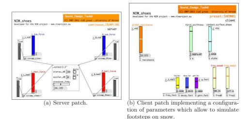
Fig. 3.10. Patches for Pd which use the *continuous-crumpling* model in order to render audio-haptic cues of footsteps on aggregate grounds.
