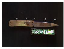
(b) The knife, opened up in order to show the embedded board which is taken from a Wii Remote controller.
