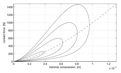
Fig. 1.2. Compression-force characteristics for varying input velocities:  $v_{\rm in} = 1 \dots 4$  m/s. Solid lines represent the case when dissipation is taken into account (the values of parameters are the same as in Fig. 1.1), while the dashed line represents the curve  $kx^{\alpha}$ , where no dissipation is considered ( $\lambda = 0$ ).
