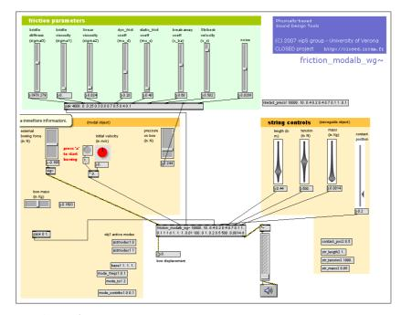
**Fig. 2.4.** A Max/MSP patch implementing the contact interaction between two solid objects. The object in the center, which is named friction\_modalb\_wg~ and takes several inputs from sliders or other control devices, is the graphical representation of the corresponding homonym *external* implementing the friction between a modal and a waveguide resonator.
