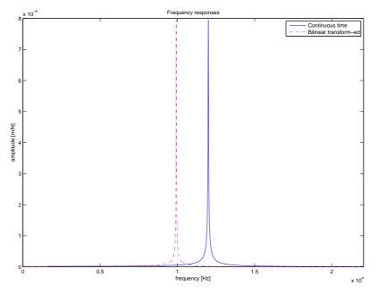
Fig. A.1. Frequency responses of a continuous-time and bilinear transform-ed harmonic oscillator having natural frequency  $\omega = 12000$  Hz, damping coefficient g = 166.6667 Hz and modal mass m = 0.001 Kg. The sampling frequency is  $F_s = 44.1$  kHz. The effect of warping is clearly evident: the frequency of the discretized oscillator is  $\omega_{BT} = 9928.78$  Hz.
