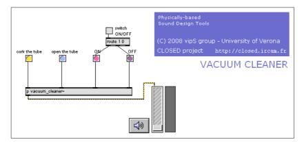
Fig. 2.16. The Max/MSP patch implementing the vacuum cleaner model.
