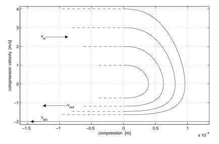
Fig. 1.1. Phase portraits for varying input velocities:  $v_{\rm in} = 1...4$  m/s. Other values of parameters are:  $m = 10^{-2}$  kg,  $k = 10^9$  N/m<sup> $\alpha$ </sup>,  $\mu = 0.5$  s/m,  $\alpha = 1.5$ . Solid lines represent the trajectory of the mass during contact; dashed lines represent free motion.
