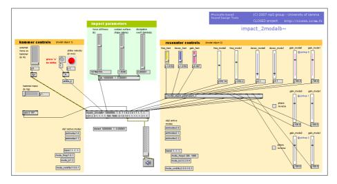
**Fig. 2.3.** A Max/MSP patch implementing the contact interaction between two solid objects. The object in the center, which is named impact \_2modalb~ and takes several inputs from sliders or other control devices, is the graphical representation of the corresponding homonym external implementing the impact between two modal resonators.
