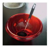
(d) The tureen lays on a magnetic field sensor, while two thin magnet stripes are glued to the bottom of the ladle, thus providing data as the ladle moves inside the tureen.
