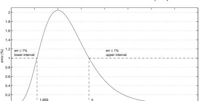
Fig. 1.3. Percentage error on the output velocity introduced by  $\tilde{v}_{out}$  with respect to the value computed numerically as a zero of (1.6). As an example, the ranges of  $\mu v_{in}$  are shown, for which the maximum error is equal to 1% (see Table 1.1).
