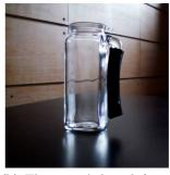
(b) The jug. A board from a Wii Remote is embedded into the handle and covered with rubber.
