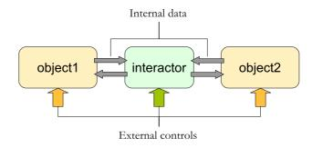
Fig. 2.2. The common structure underlying the SDT's algorithms simulating solid contacts.
