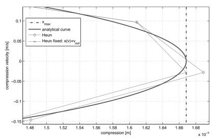
Fig. 1.9. Detail of phase portrait of Heun-based simulations with and without correction (the compression x is forced to  $x_{\text{max}}$  when exceeded). The values of parameters are  $k = 10^7 \text{ N/m}^{\alpha}$ ,  $\mu = 0.1 \text{ s/m}$ ,  $\alpha = 1.1$ ,  $v_{\text{in}} = 0.3 \text{ m/s}$ .
