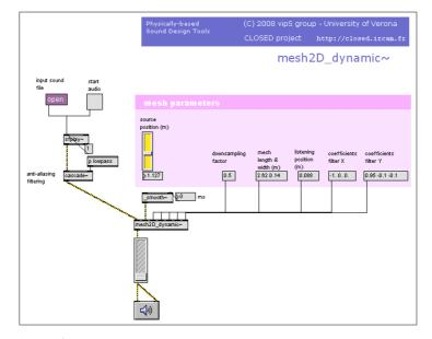
Fig. 2.6. A Max/MSP patch making use of the DWM spatialization model, implemented as the *external* named mesh2D dynamic~.
