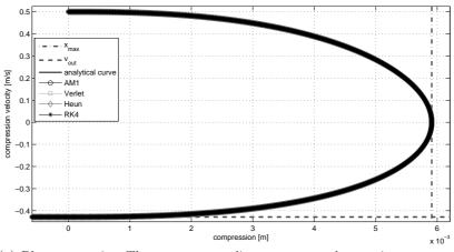
(a) Phase portraits. The two tangent lines represent the maximum compression  $x_{\text{max}}$  calculated by (1.4) and the output velocity  $v_{\text{out}}$  computed numerically as a zero of (1.6).
