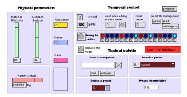
Fig. 2.21. High-level interface for the impact model: physical parameters, temporal control and timbral palette sections.
