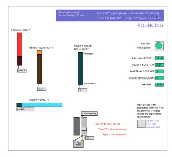
Fig. 2.8. Example patch for Max/MSP implementing the high-level bouncing model.
