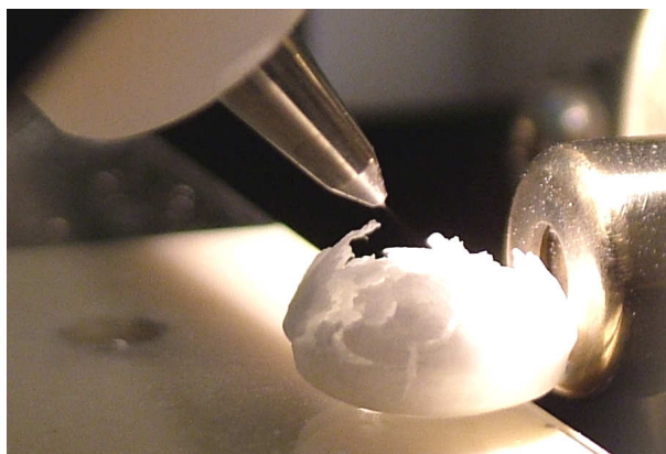
Figure 50. Fall apart and break of Acetylsalicylic Acid tablet after test with water/methanol mixture
