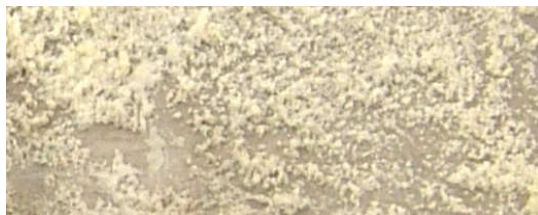
Figure 64. 4-methyl-7-hydroxycoumarin crystals deposited on cyanoacrylic resin
