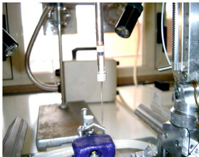
Fig. 11. In house injection system with glass micropipette used for viral vectors injection.
