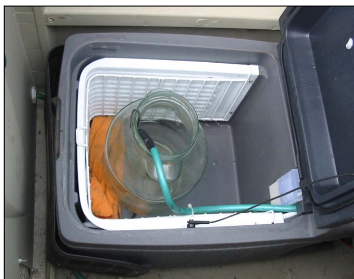
Figure 5.1. Classical portable automatic sampler
