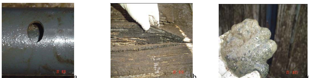
Figure 8.6 a-b-c. Aeration system for membrane scouring (a) and membrane clogging (b, c) caused by excess of grit in the activated sludge
