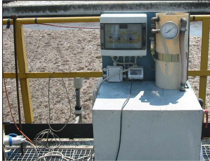
Figure 5.2 Special automatic sampler used to separate liquid from solid phase
