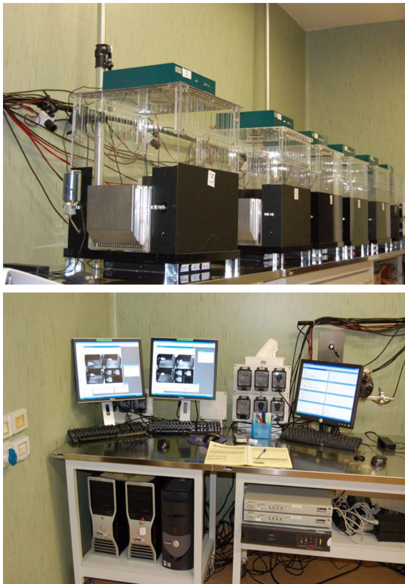
Figure 4: The final EEG-video-telemetry system installed in our laboratory.
