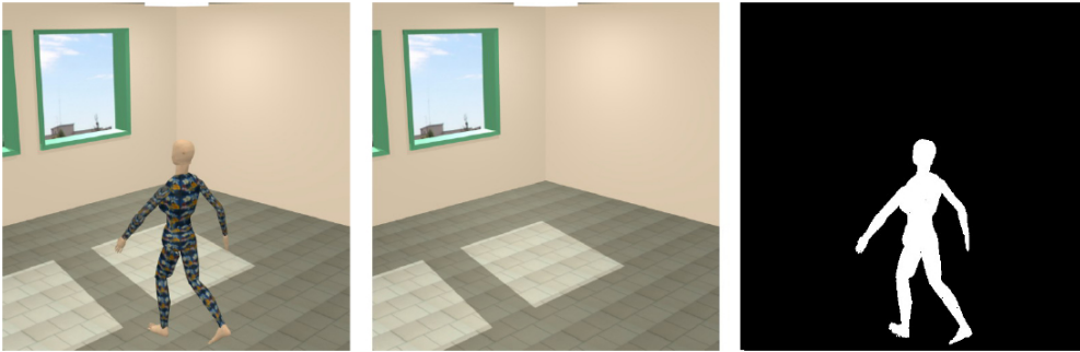
Fig. 3.1. The foreground/background subtraction phase using a virtual room created using Blender.
