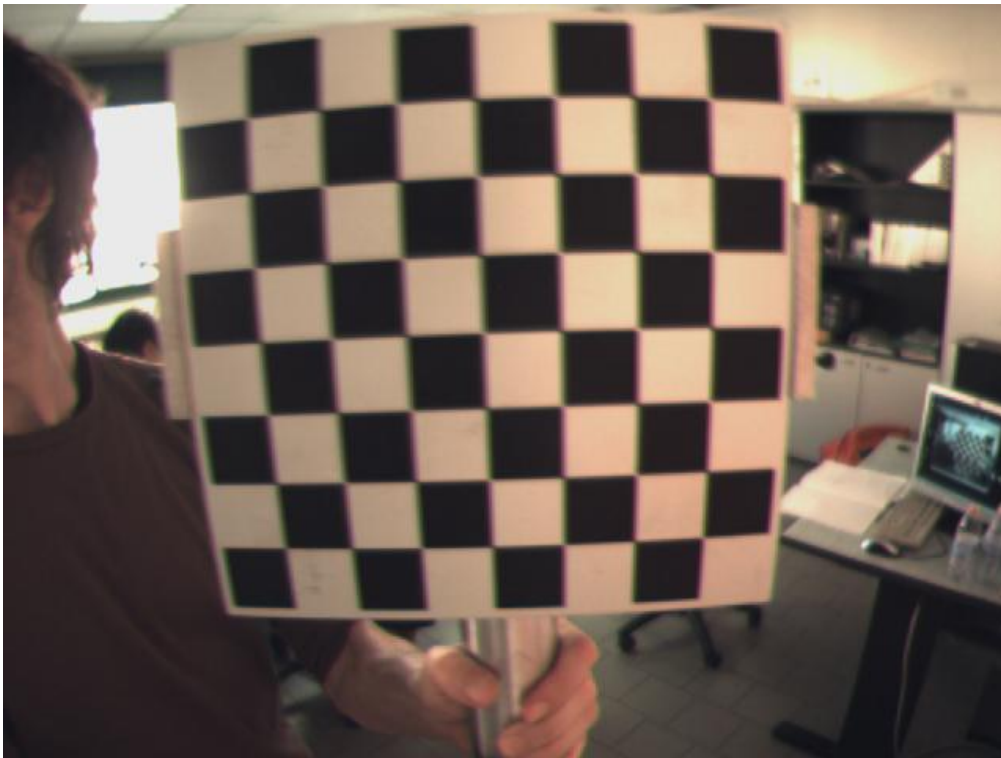
Fig. 6.1. The checkboard used for the intrinsic camera parameters.
