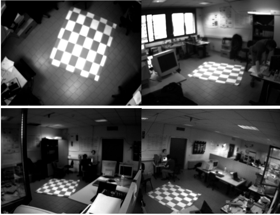
Fig. 6.3. The calibration checkboard used for the extrinsic camera parameters computation. Note that in these images there still be distortion due to the camera lens.
