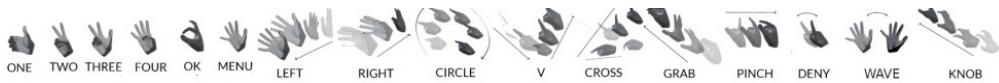
Fig. 6. The 16 static and dynamic gestures modeled in [9] that are used for touchless control.
