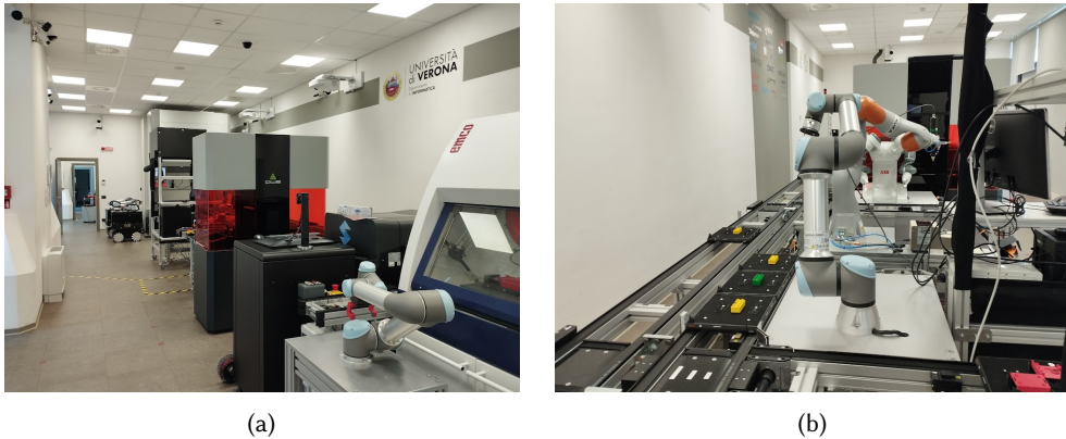
Fig. 1. Two views of the ICE laboratory: (a) shows the milling machine close-by with the feeding arm in the forefront, the polyjet and stereolithographic printers in the middle, the autonomous ground vehicles and the vertical automated warehouse at the back; (b) shows the mini-pallet conveyor line on the left and the robotic arms in the middle.
