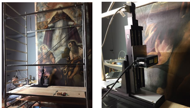
Figure 2. Scanning profilometry on the Tintoretto masterpiece Saint Martial in Glory , altarpiece from the church of San Marziale in Venice (Italy). The conoscopic holography sensor is mounted on micrometric stages to scan the painting in the vertical plane at safe working distance.
