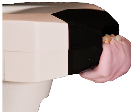
Figure 2. Silicone support used to accommodate the dental elements for the spectrophotometric analysis.
