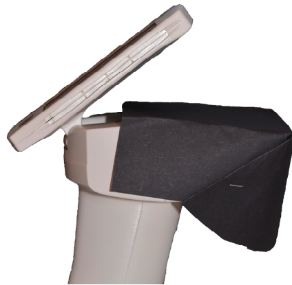
Figure 3. Black cardboard used around the spectrophotometer sensor to simulate the “oral cavity void”.
