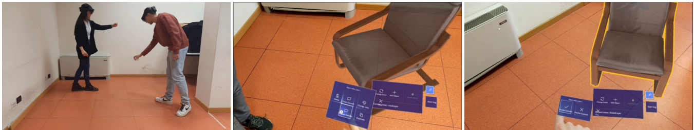
Figure 1: Left: two subjects wearing the HoloLens 2 and using CIDER in our lab. Center: one of them places a virtual chair in the room and proposes the update of the global scene with a two-phase commit operation. Right: The other subject receives a notification and can see the proposed scene, accepting or refusing the global update. The internal views are directly recorded from the apps.
