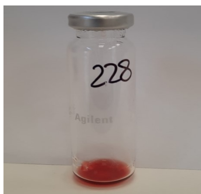
Figure 6: Headspace analysis glass vial containing the solution to be analyzed (sample + IS).
