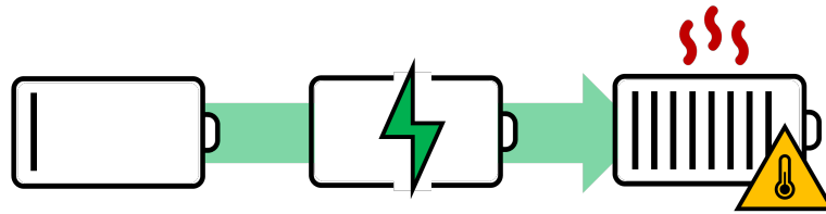
(a) Battery overheats while charging.
