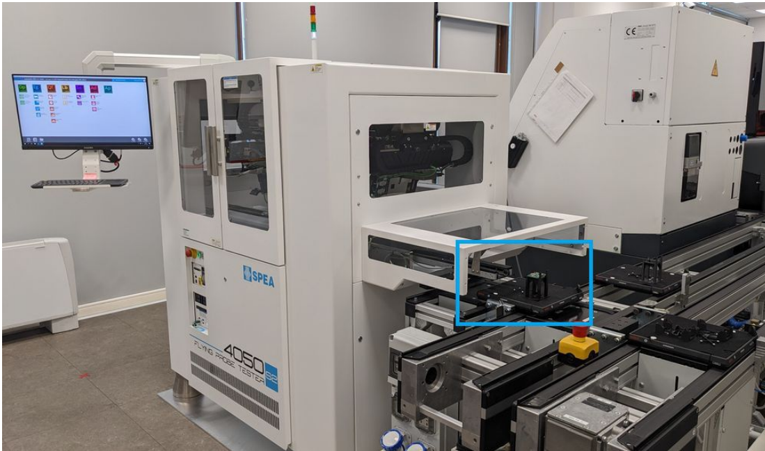
Fig. 4.29: The SPEA 4050S2 Automatic Flying Probe Tester in the ICE Laboratory. The highlighted area shows a mini-pallet sliding toward the side bay to position a board for testing and programming.
