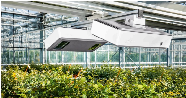
Figure 6.12: Phenospex 3D scanning system for high-precision plant trait measurement under controlled environments.
