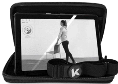
Fig. 1. The figure illustrates the technological solution consisting of a tablet (the dedicated software displays video instructions and real-time visual feedback) and a wearable inertial sensor (magnetically attached to an elastic band).
